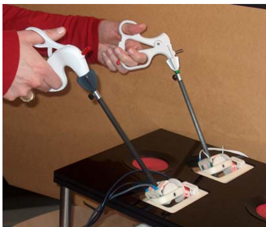
Fig. 2 TrEndo tracking system to measure laparoscopic instrument movements in a box trainer
