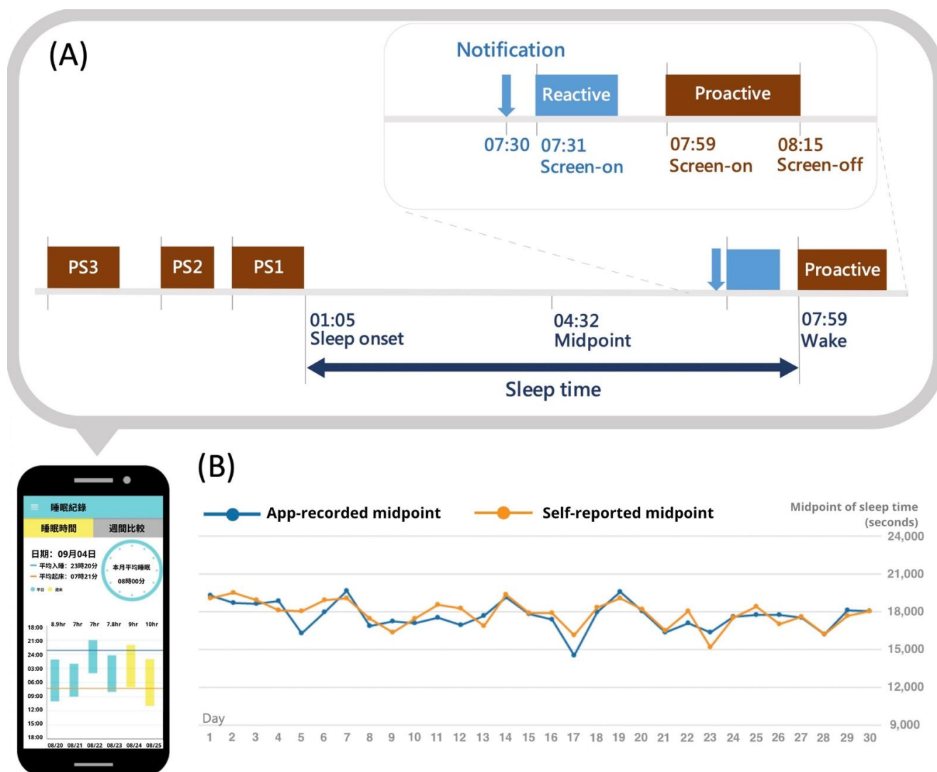
Figure 4. (A) Smartphone use from screen-on to the successive screen-off was defined as one episode of use. Usage episodes without notifications during the one minute before screen-on were classified as proactive use, whereas episodes with notification during the one minute before screen-on were classified as reactive use. Only proactive use episodes were included in the calculation of sleep time. (B) Daily app-recorded and self-reported midpoints of sleep time were compared to validate the fluctuations in circadian rhythms. The figure showed a high agreement between app-recorded and self-reported midpoints of sleep time.
