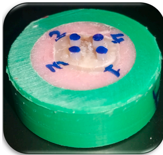
Figure 1. Four macroshear cylindrical composite samples bonded to dentinal substrate.
