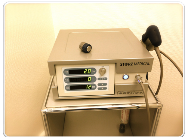
Fig. 4. The Storz Medical Masterpuls® MP 100 radial shock-wave system with a trigger point applicator was used in this study
