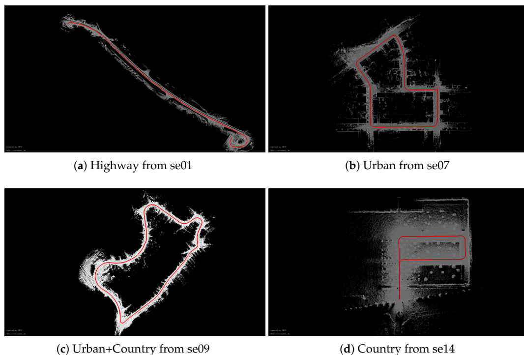
Figure 15. The point-cloud map of four experiments, which is calculated by SE+PTP+6DSLAM. The red line is the trajectory of the vehicle. (a) se01. (b) se07. (c) se09. (d) se14.
