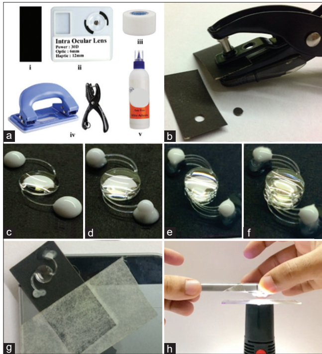
Figure 1: (a) Materials used to prepare IOLSCOPE; i. Black chart paper strip measuring 4 cm × 2 cm, ii. Intraocular Lens - 30D four in number, iii. Micropore, iv. Paper punching machine, v. Liquid adhesive, (b) Circular opening of 5 mm made on one end of the black strip using the punching machine, (c-f) Placing the first IOL on the circular hole and the subsequent IOL's one upon the other by applying liquid adhesive, (g) Placing the optical device on the camera of the smartphone using micropore, (h) Placing the slide on a light source (torch) and taking pictures by approximating the iolscope to it
