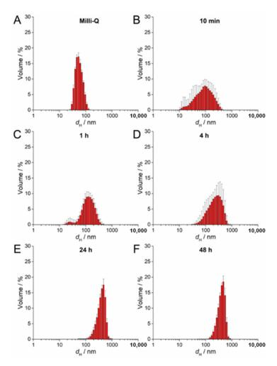
**Figure 3.** Size distribution plots of 100  $\mu$ M AgNP-PVP in (**A**) ultrapure water and after (**B**) 10 min, (**C**) 1 h, (**D**) 4 h, (**E**) 24 h, and (**F**) 48 h in exposure solution (liquid 1/2 strength MS medium).
