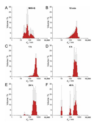
**Figure 4.** Size distribution plots of 100  $\mu$ M AgNP-CTAB in (**A**) ultrapure Q water and after (**B**) 10 min, (**C**) 1 h, (**D**) 4 h, (**E**) 24 h, and (**F**) 48 h in exposure solution (liquid ½ strength MS medium).
