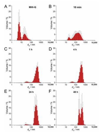
**Figure 2.** Size distribution plots of 100  $\mu$ M AgNP-citrate in (**A**) ultrapure water and after (**B**) 10 min, (**C**) 1 h, (**D**) 4 h, (**E**) 24 h, and (**F**) 48 h in exposure solution (liquid ½ strength MS medium).
