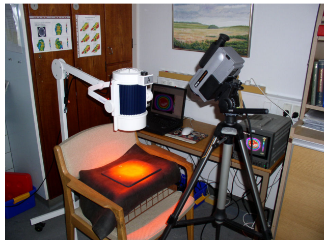
Figure 2: Experimental set-up for testing a wIRA radiator The photograph shows a porous rubber mat being heated by a wIRA radiator. The surface temperature of the irradiated porous rubber mat is continuously monitored by the infrared camera.
