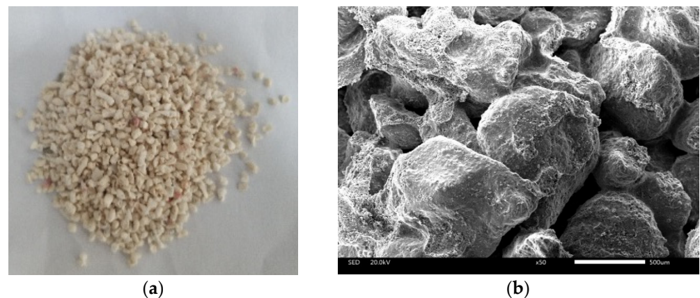
Figure 1. Particle morphology of coral sand: (a) picture of coral sand; (b) SEM image with 50\times magnification.
