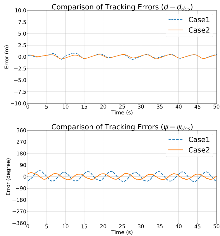
Figure 10. Simulation 1: Comparisons of the state vector tracking errors.
