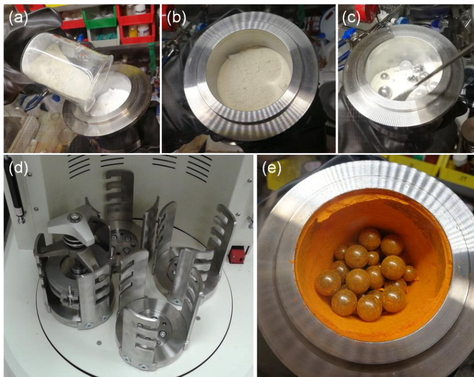
Figure S3. Photographic demonstration of the kg-scale synthesis of \text{CsSnBr}_{1.5}\text{Cl}_{1.5} . a) Preparation of the reagents \text{CsBr} , \text{CsCl} , \text{SnBr}_2 , and \text{SnCl}_2 (all white powders) in a \text{N}_2 glovebox. The reagents were weighed and transferred from a beaker into the 250 mL mechanochemical reaction vessel. The total reagent weight was 250 g. b) The reagent mixture with the milling balls at the bottom of the vessel. c) Gentle mixing of the reagents, which exposed the milling balls, by using a metal spatula. d) Planetary mill containing four reaction vessel holders, essentially allowing four 250 g reactions to take place simultaneously, leading to a 1.0 kg scale batch synthesis of the perovskite. e) The orange product after 10 hr of milling. Related to Figures 1 and 4.
