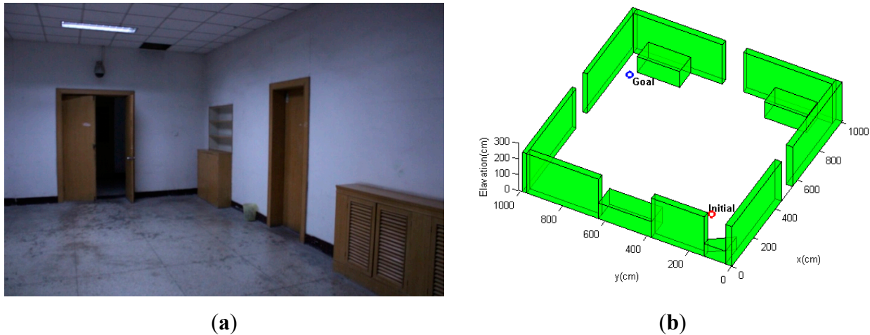
Figure 7. Indoor environment simulation Scenario 1: (a) A hallway of Tsinghua University’s main building; (b) simulated 3D model of the GPS-denied indoor environment. The red and blue circles indicate the initial and goal location of the MAV, respectively.
