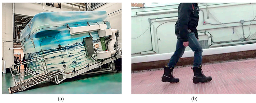
Figure 1. WinterLab at the KITE Research Institute (a) outside view and (b) inside view (glycol pumped through tubes below the ice surface).
