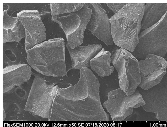
Figure 2. SEM image of SAP powders.
