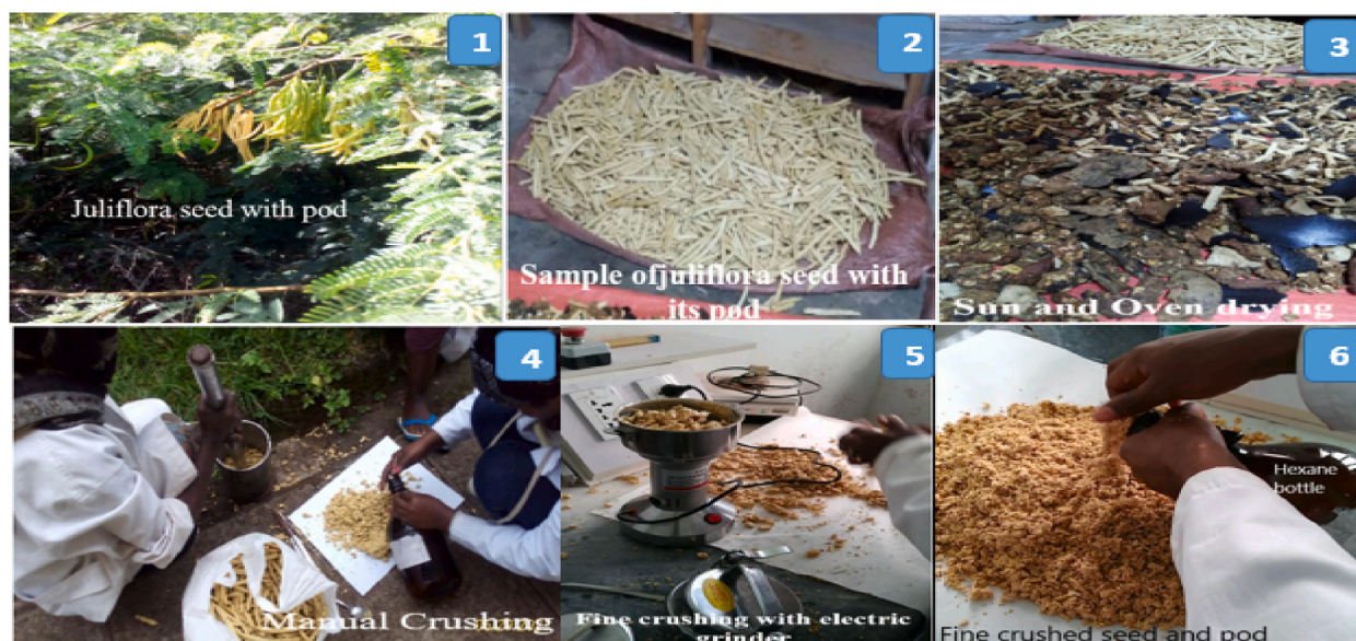
Fig. 2. Preparation phases of juliflora seed (1. juliflora fruit, 2. juliflora seedpod, 3. Sun drying Process, 4. mechanical crushing, 5. fine crushing with electric grinder, 6. crushed seed powder collection).
