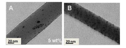
Hydrophilic nylon-6 is one of the famous electrospinning membrane materials [45]. Accordingly, Park *et al.* [29,71] developed nylon-6 nanofibers (150–250 nm in diameter) containing well dispersed silver nanoparticles. Such a nanocomposite ENM showed an optimized antibacterial activity as compared to its neat counterpart thereby a high potential as a water filtration membrane.
