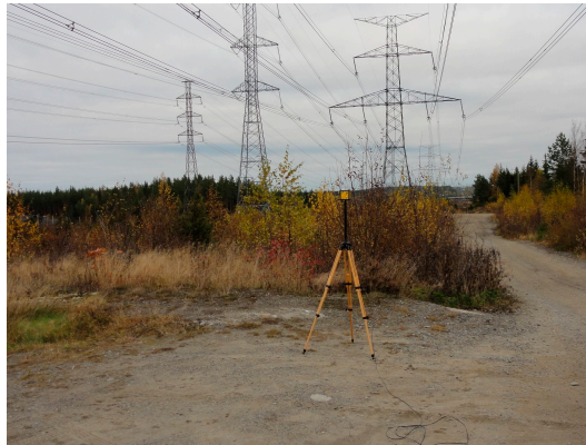
Figure 2. Electric field measurement at experiment location.
