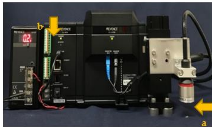
Figure 1. Multicolor confocal displacement laser used in this study for measuring the shrinkage of short fiber reinforced composites. (a): a center head CL-L007G, Keyence, Osaka, Japan, (b): optical unit CL-L015, Keyence, Osaka, Japan.
