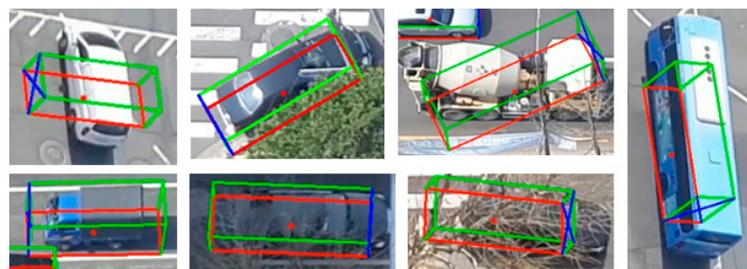
**Figure 11.** Examples of inaccurate vehicle 3D box estimates based on DCNN models.
