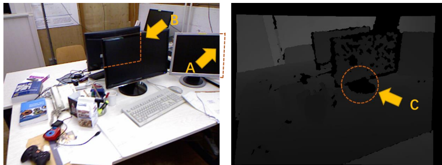
Figure 3. Classic challenges of RGB-D observations. (A) Occlusions by image edges; (B) occlusions by objects; (C) invalid depth values.
