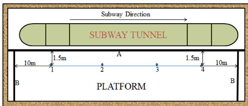
A: Full-height safety door or shielding door      B: Isolation door
