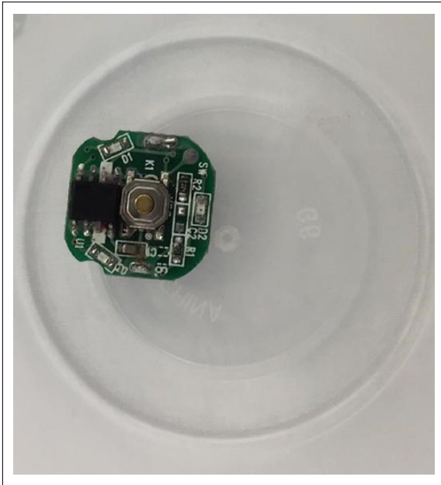
Figure 3. Picture of foreign body showing the fidget spinner's circuit board with metallic components and sharp edges.
