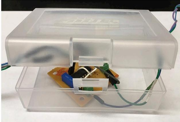
**Figure 5. Enclosure to Protect Circuit Wiring**
