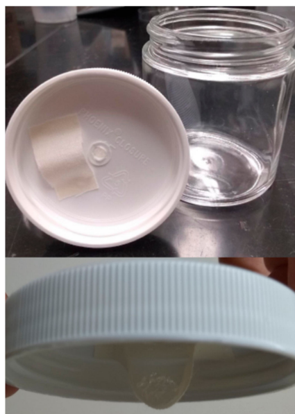
Figure 1. Thrips fumigation chamber with hydrogel “pouch”.
