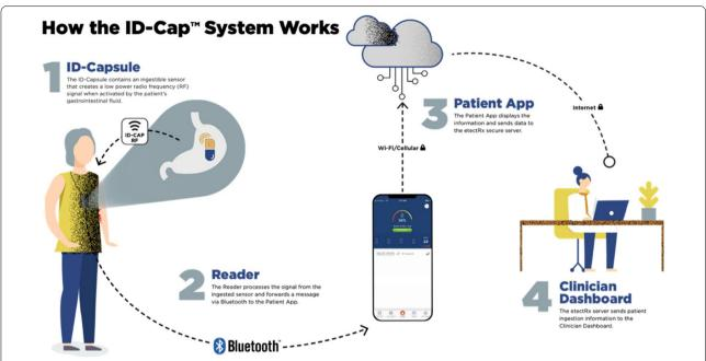
Fig. 1 Overall functionality of the US Food and Drug Administration (FDA)-cleared etectRx ID-Cap System, the digital pill system (DPS) utilized in this study. Image courtesy of etectRx
