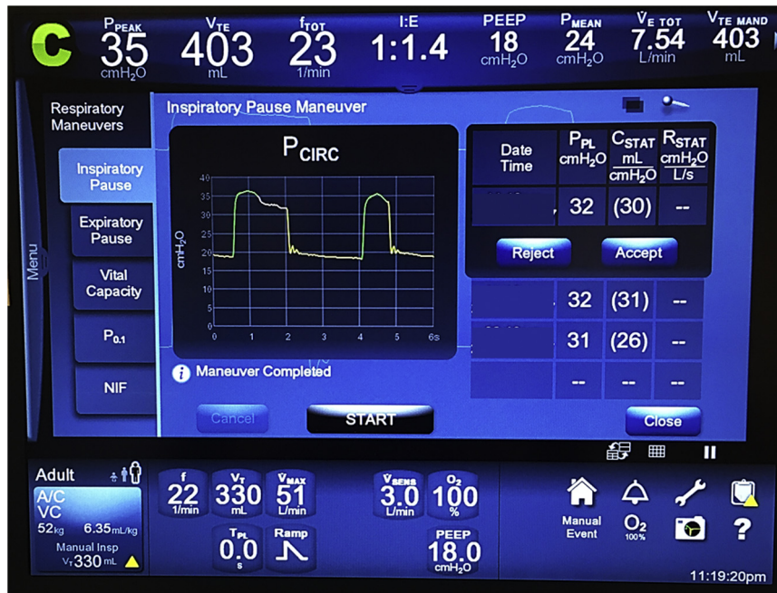
Figure 3. An inspiratory hold maneuver on a ventilator, showing a peak inspiratory pressure of 35 cm H 2 O and a plateau pressure of 32 cm H 2 O, on a tidal volume of 330 mL and 18 cm H 2 O of positive end-expiratory pressure.
