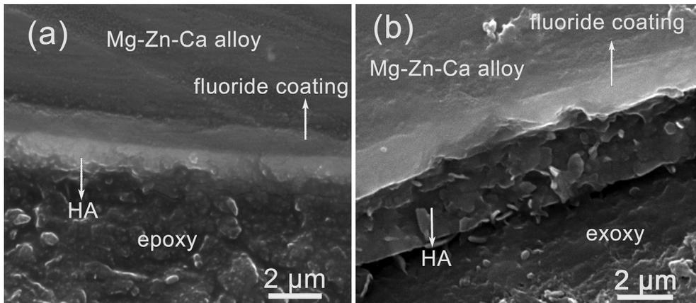
Fig. 6. The cross-section image of (a) PRC-HA/MgF<sub>2</sub> and (b) TED-HA/MgF<sub>2</sub> composite coating on Mg-Zn-Ca alloy.
