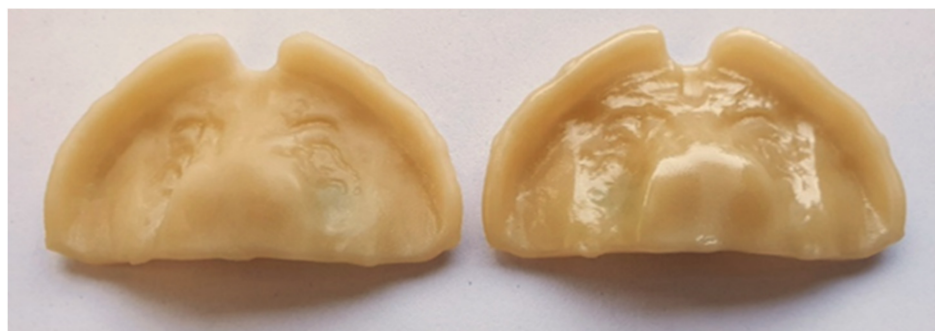
Figure 7. Difference of surface finishing between Yamahachi PMMA blanks after manufacturing. Left: manufacturing after PEEK blanks and used tools. Right: manufacturing with new tools.
