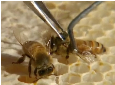
Figure 3. RFID tag being fitted to the thorax of a honey bee. This process can be done in the hive with non-aggressive bees.
