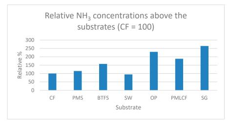
Figure 4. NH<sub>3</sub> concentrations measured above the individual substrates at day 8.
