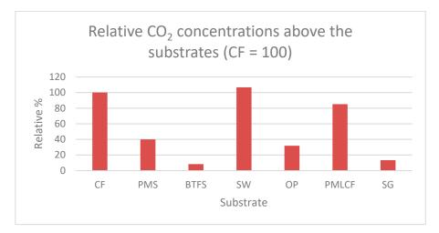
Figure 3. CO<sub>2</sub> concentrations measured above the individual substrates at day 8.
