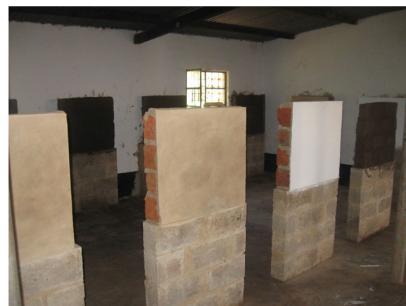
Fig. 1 Experimental walls (approximately 0.5 m 2 ) showing left to right surfaces of cement, painted cement, and unbaked clay (baked clay surface not shown)
