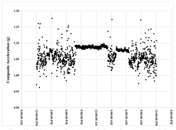
**Figure 3.** MicroPEM composite acceleration time series that illustrates the participant's activity level and 89% compliance wearing the device according to the study protocol.
