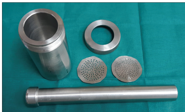
Figure 6: Hand operated order made stainless steel apparatus and sieves of size: 500, and 1200 nm
