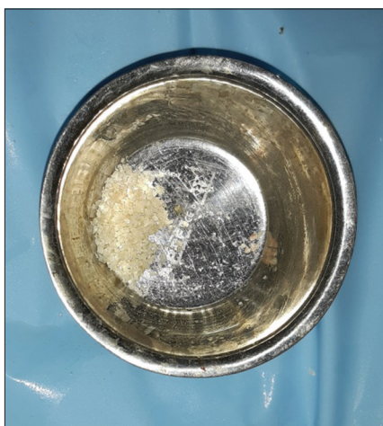
Figure 7: Crushed tooth particulate of particle size ranges from 500 nm to 1200 nm
