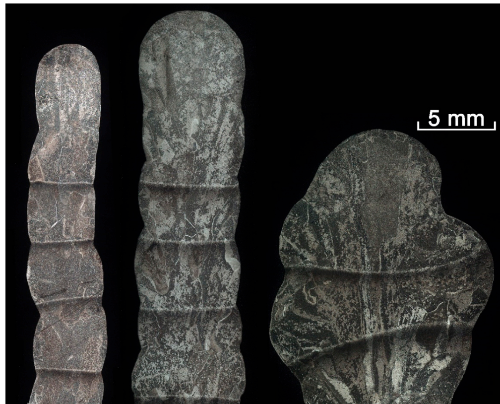
Figure 12. Walls: CMT—on the left, CSC—in the center, DCEN—on the right.
