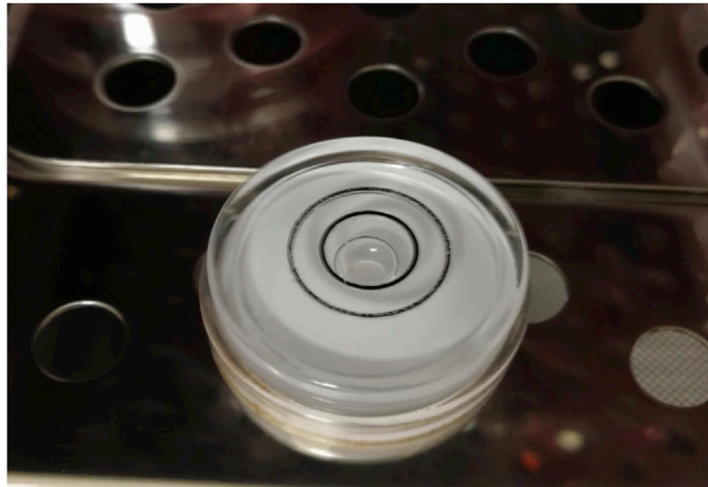
Figure 2. Measurement of cell incubator balance using a spirit level
