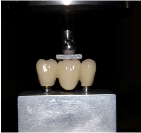
Fig. 2: Position of stainless steel ball and Teflon disk at loading point
