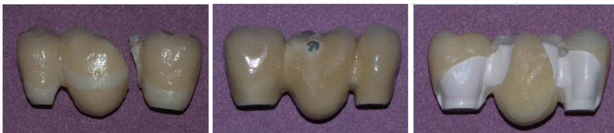
Fig. 3: Examples of a fractured FPD (left to right: zirconia, metal ceramic and PEEK restorations)
