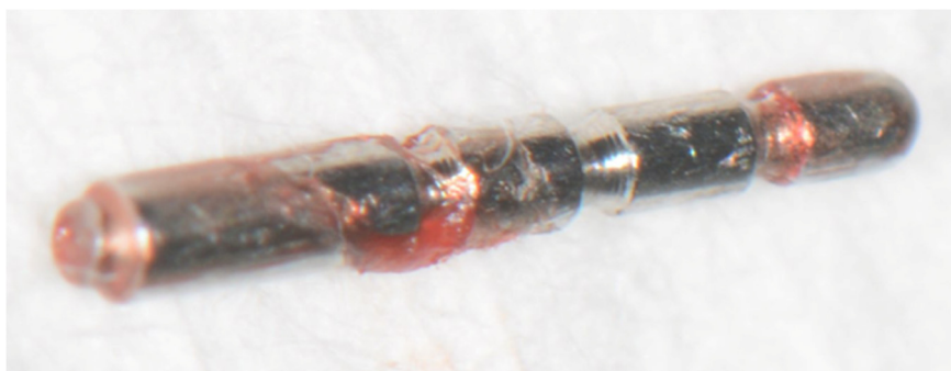
Figure 6. The surgically removed fragment tip of a periodontal probe type AE P OWP.
