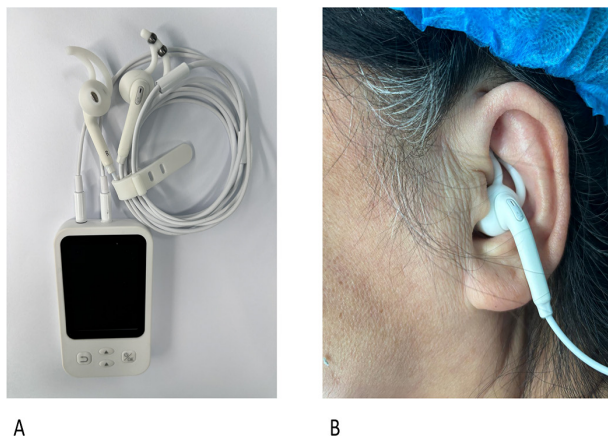
Figure 2 (A) Stimulation device (tvNS501, RISHENA). (B) Stimulation location of transcutaneous auricular vagus nerve stimulation.
