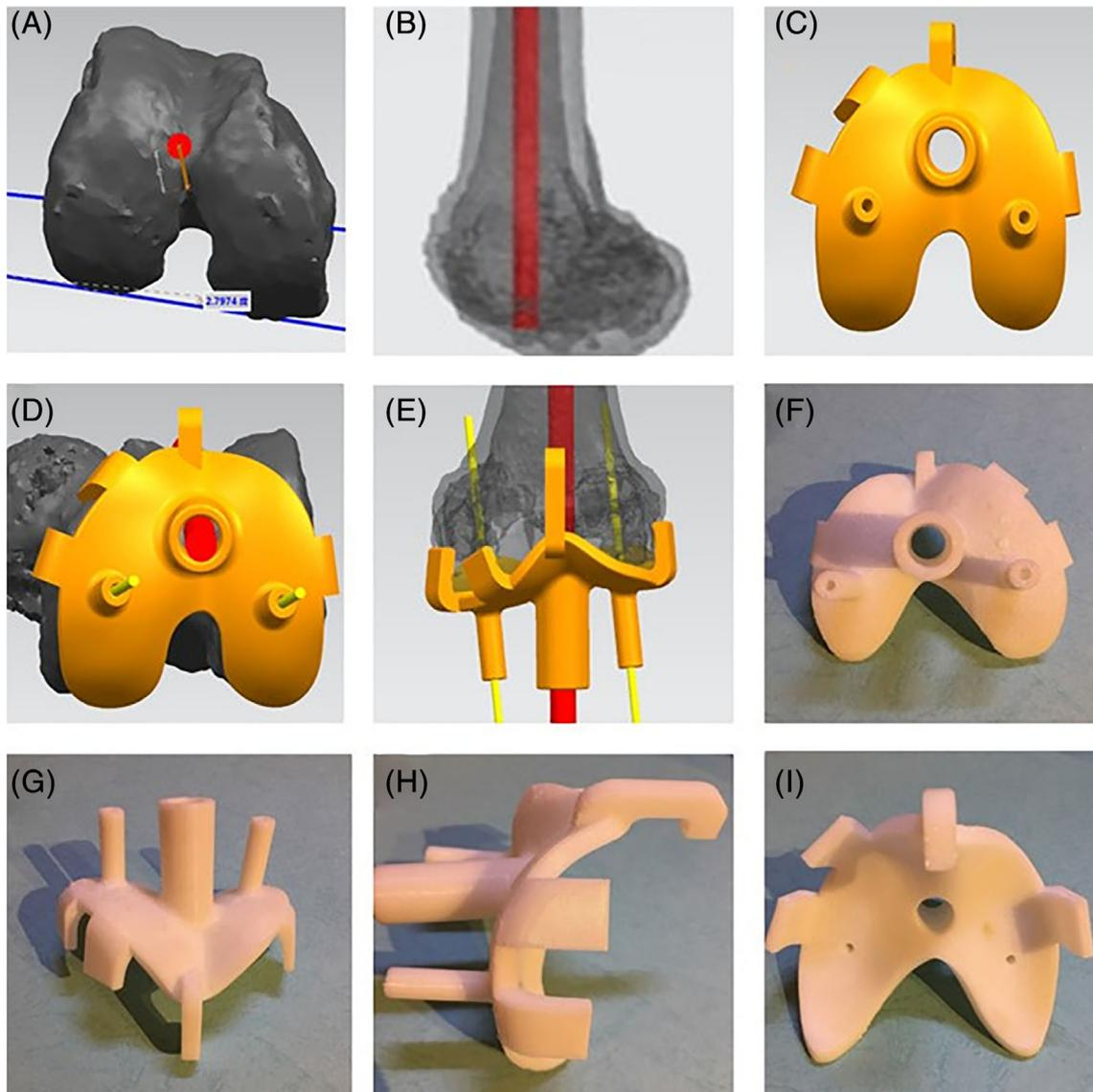
**Fig. 2** The process of designing PSI and the morphology of the PSI:(A, B) Finding the sTEA and the location of intramedullary guide; (C–E) The process of designing PSI; (F–I) The morphology of PSI in different perspectives.
