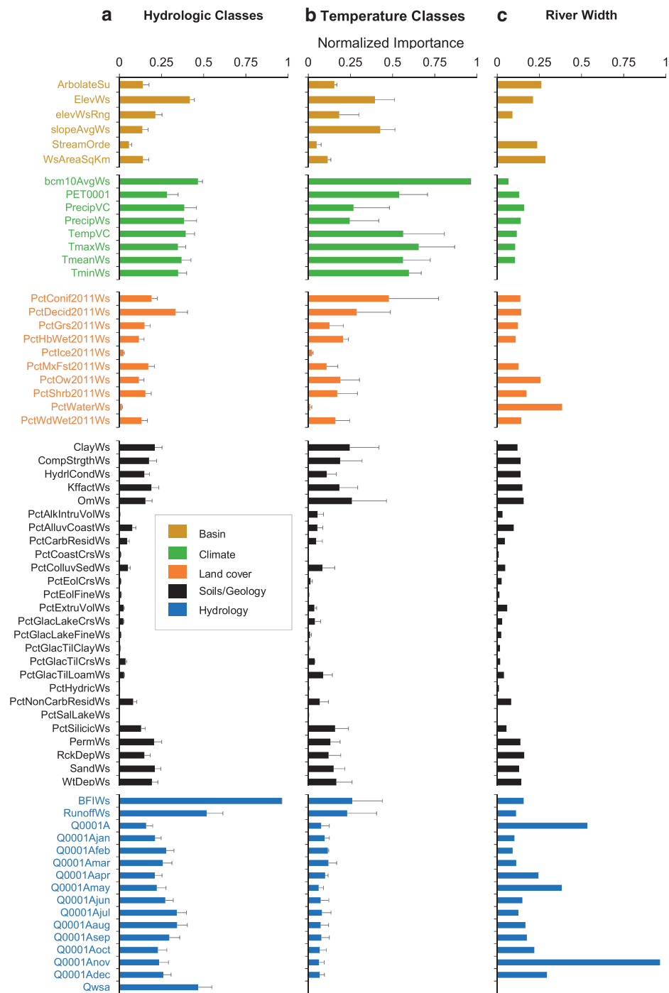
Figure 4. Importance of different predictors used in random forest models. Random forests were used to predict (a) hydrologic classes, (b) temperature classes or average July–August temperature, or (c) river width. Normalized importance refers to node impurity values for the Gini index (classification) or mean-squared error (regression) that are scaled from 0 to 1 using (\max - x_i)/(\max(x) - \min(x)) . Normalized importance was averaged across all random forest models for hydrologic classes and temperature. Error bars represent 1 SE. Note: only 1 random forest model was developed for river width.
