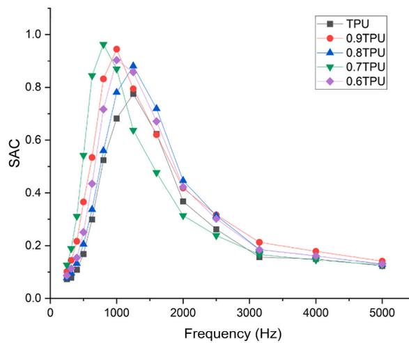
Fig. 17. Effect of the OPTD loading on the sound absorption coefficient (SAC) of TPU (without air gap).
