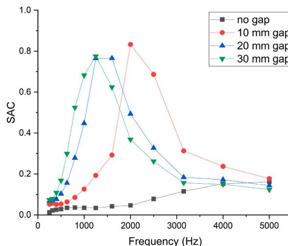
Fig. 18. Effect of air gap to the sound absorption coefficient of the TPU samples.
