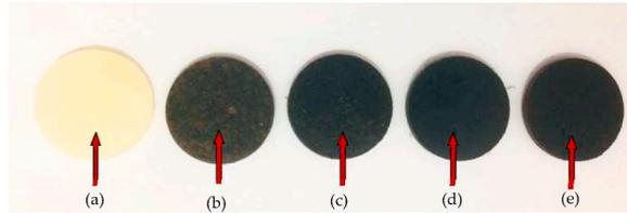
**Fig. 2.** Fabricated (a). PU, (b). 0.9 TPU, (c). 0.8TPU, (d). 0.7TPU, and (e). 0.6TPU samples.
