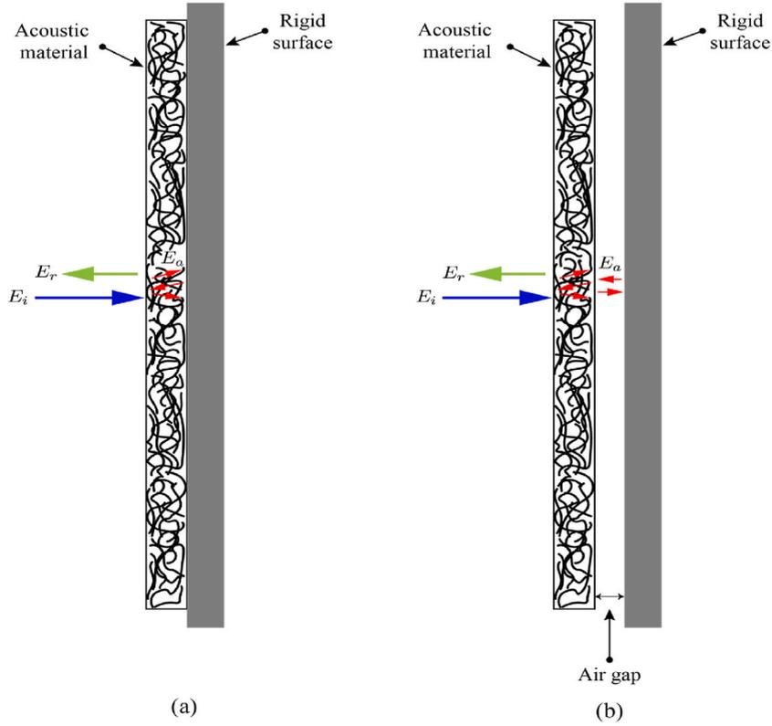
**Fig. 4.** Illustration of sound absorption mechanism in an acoustic material: (a) without air gap and (b) with air gap.
