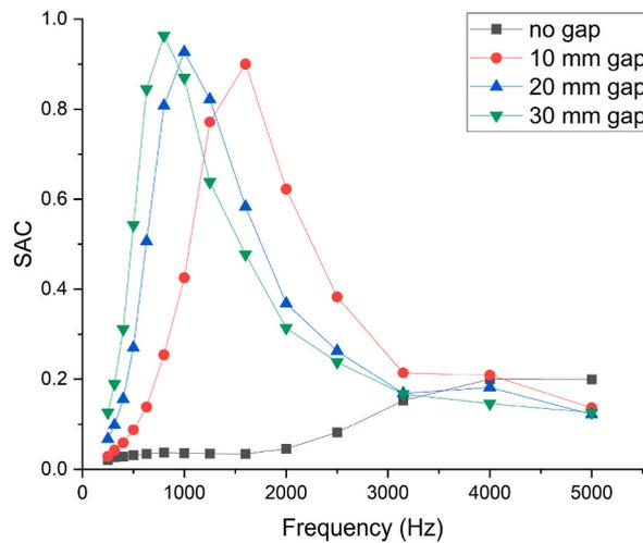
Fig. 21. Effect of air gap to the sound absorption coefficient of the 0.7TPU samples.
