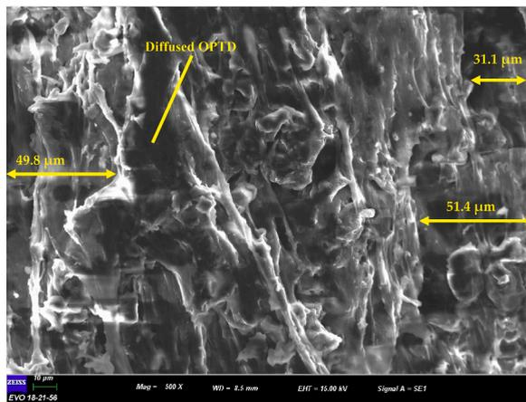
Fig. 16. Microstructure of 0.6TPU sample (500×).
