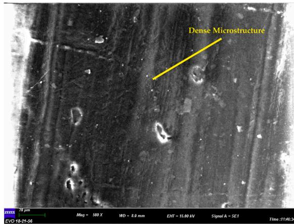
Fig. 12. Micrograph of TPU sample (500 × ).
