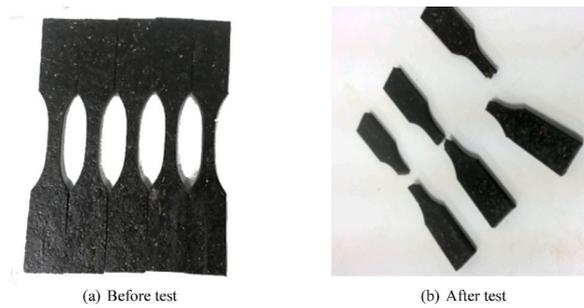
Fig. 10. The samples before and after the tensile test.
