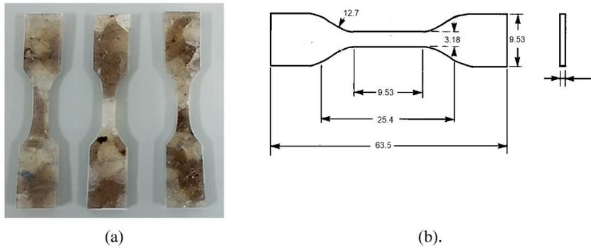
**Fig. 3.** Fabricated tensile test sample (a) and its relative dimension (b).
