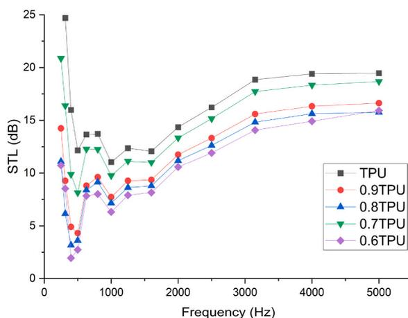
Fig. 23. Effect of OPTD loading on sound transmission loss (STL) of the test samples.
