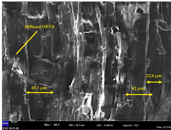
Fig. 15. Microstructure of 0.7TPU sample (500×).
