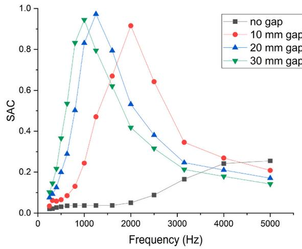
Fig. 19. Effect of air gap to the sound absorption coefficient of the 0.9TPU samples.
