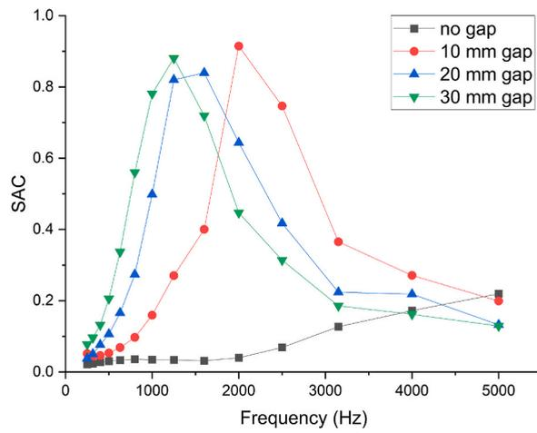
Fig. 20. Effect of air gap to the sound absorption coefficient of the 0.8TPU samples.
