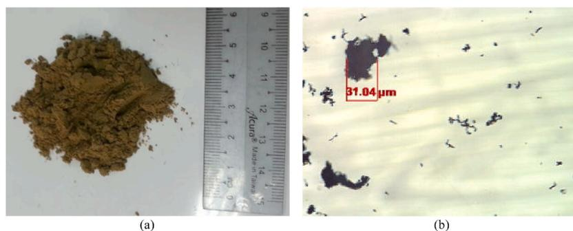
Fig. 1. Oil palm trunk dust (OPTD) sample. (a) OPTD sample after filtered, (b) micro-photograph of OPTD sample (100 × Mag.).
