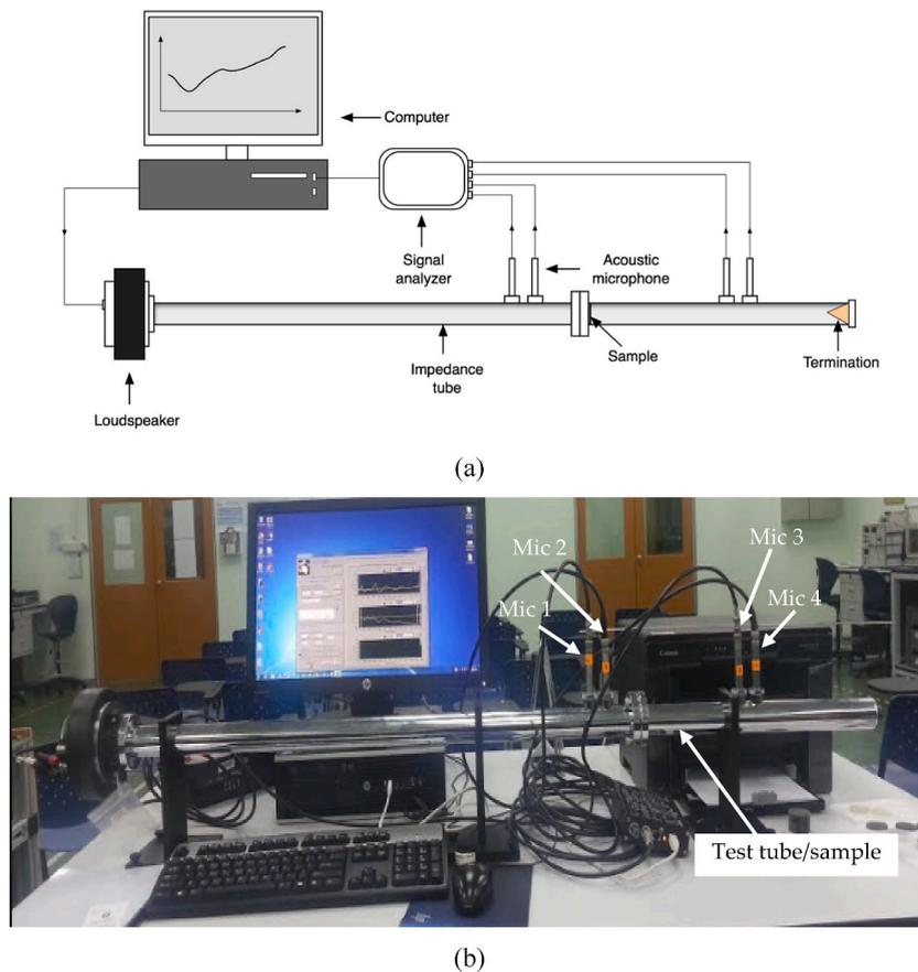
**Fig. 7.** (a) Schematic diagram and (b) Photo experimental setup for sound transmission loss.
