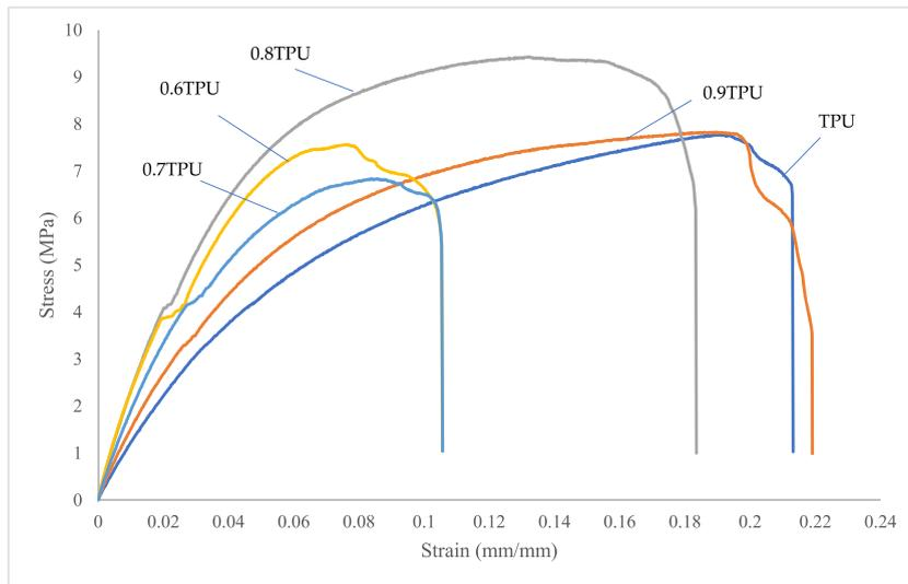
Fig. 9. Typical stress-strain curve obtained from tensile test.
