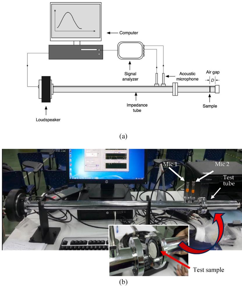
Fig. 5. (a) Schematic diagram of experiment set up, and (b) Photo of the experimental setup.
