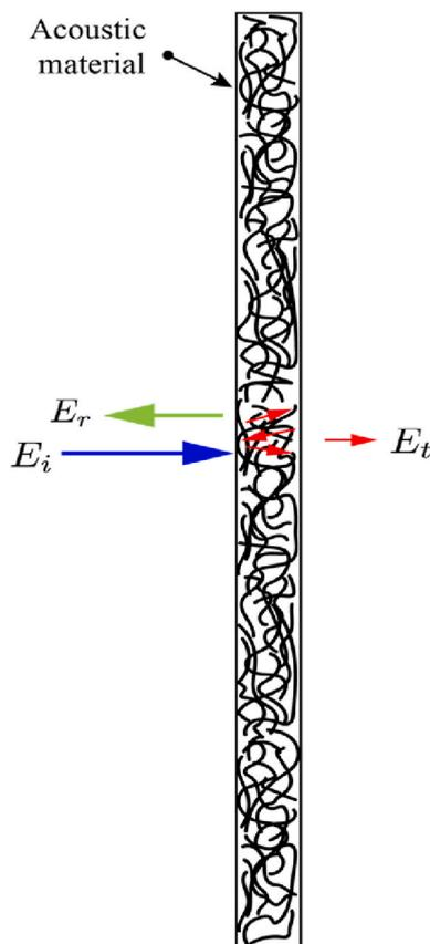
Fig. 6. Illustration of sound transmission through a partition.
