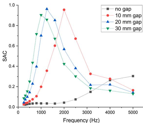
Fig. 22. Effect of air gap to the sound absorption coefficient of the 0.6TPU samples.
