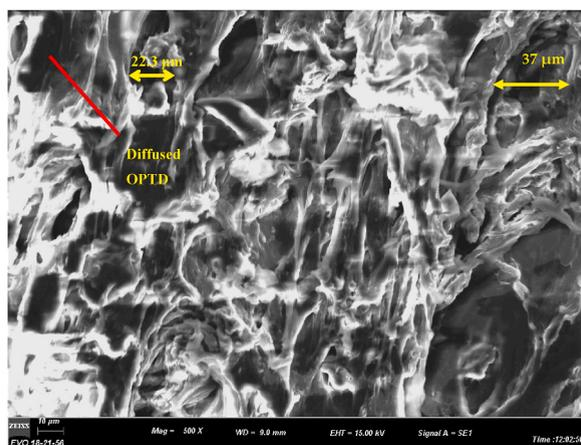
Fig. 14. Microstructure of 0.8TPU sample (500 × ).
