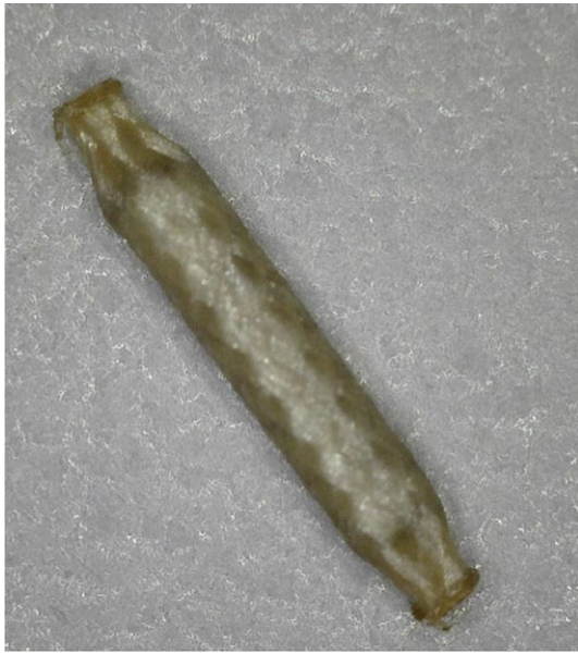
Fig. 1. Braided vicryl seed encapsulation used with AgX100 seed as used in this study. The nominal seed length before encapsulation is 4.5 mm.
