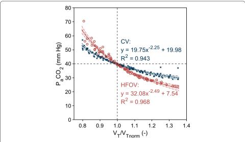
**Fig. 1** Stronger effect of tidal volume changes on  $CO_2$  elimination during high-frequency oscillatory ventilation (HFOV) compared to conventional mechanical ventilation (CV) close to normocapnia. Tidal volume is presented as relative to normocapnic tidal volume  $V_{T \text{ norm}}$ . Fitted curves are plotted with 95% functional prediction intervals
