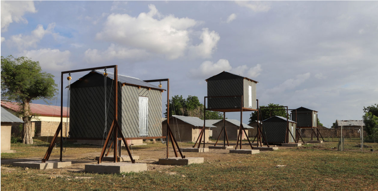
Figure 1. Experimental huts. From left to right, at 1 m, 3 m, 0 m and 2 m. Automatic weather station is shown to the right of the huts and the village to the left and rear.
