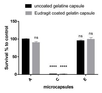
**Figure 5.** Survival compared to control (alginate uncoated microcapsules filled in uncoated gelatin capsule) of uncoated alginate (A), chitosan-coated (C), and Eudragit-coated (E) microcapsules filled in uncoated gelatin and Eudragit-coated gelatin capsule. Data are presented as means  $\pm$  SDs, n = 3. Differences were considered significant at p < 0.05; \*\*\*\* p < 0.0001, and ns means not significant.
