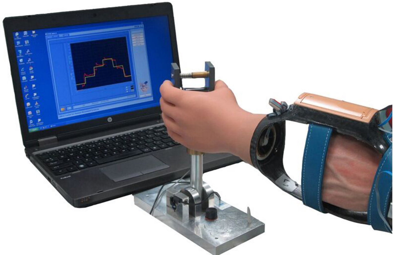
Fig 5. Force control training using the prosthesis simulator and a custom-made tracking program controlled by a handle.
