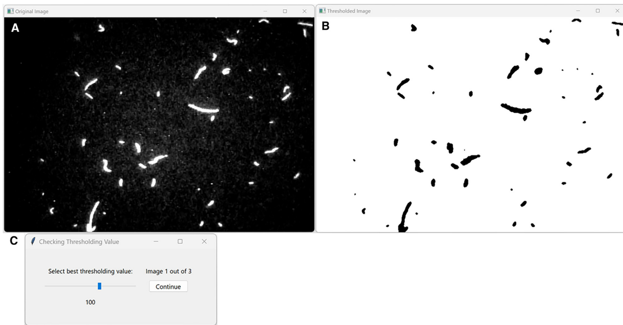
FIGURE 2 Graphical user interface (GUI) for thresholding images in Philament. When Philament is first started the user will be shown the first frame of the raw image (A), the automatic thresholded image (B), and a slider bar (C) that allows the user to adjust the thresholding value for that single image. In the case of multiple movies, Philament will randomly select 1 movie for every 50 movies imported (maximum 5 movies to threshold) for setting the thresholding values. When all images have been assessed a thresholded value, those values are then averaged, and that number is applied to all images that are analyzed.
