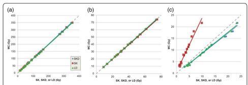
**Fig. 4** The correlation of patient absorbed doses from MC with those from LD (*green triangles*), SK (*red squares*), and SKD (*blue diamonds*) for tumor  $\overline{AD}$  (N=31) (**a**),  $NL\overline{AD}$  (N=17) (**b**), and  $RL\overline{AD}$  (N=17) (**c**) shown together with their linear fits. The *gray dashed line* represents the line of equivalence
