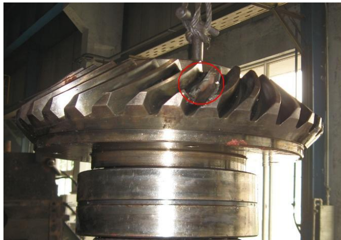
Figure 14. The real case of a broken cog fault of bevel gear Z2 (tooth 35).
