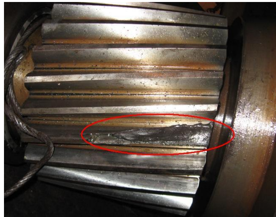
Figure 12. The real case of broken cog fault of Z5 (25-tooth) helical gear.
