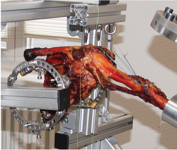
Figure 2. Human specimen in robotic test setup with the distal humerus attached to a 6-axis industrial robot (KR 60-3, KUKA). Stable scapular fixation via Schanz screws and ring fixator. Loading of rotator cuff and deltoid muscle tendons with custom-made FiberWire-construction (US 5, Arthrex) in Krakow suture technique.
